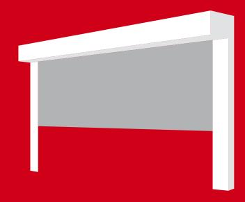
In case of fire, these curtains descend after a period of delay, isolating evacuation routes in the affected areas. Their resistance to fire and temperature is rated at E, El and EW 180-1100°C (types and temperatures). They are equipped with an irrigation system to prevent heat from radiating into the evacuation routes and making them unusable.
